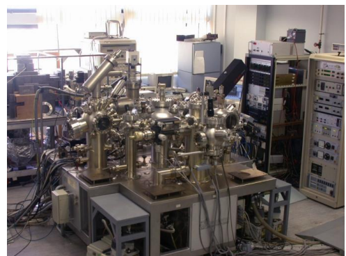
A multi-chamber ultrahigh vacuum system consisted of multi-facilities such as MBE, UPS, LEED and STM
